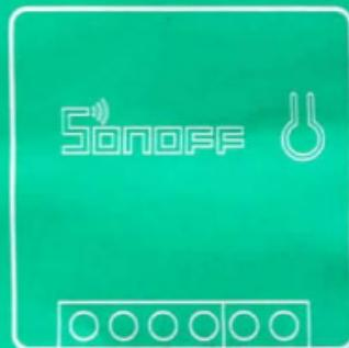
Wi-Fi Smart Switch with DIY Mode
